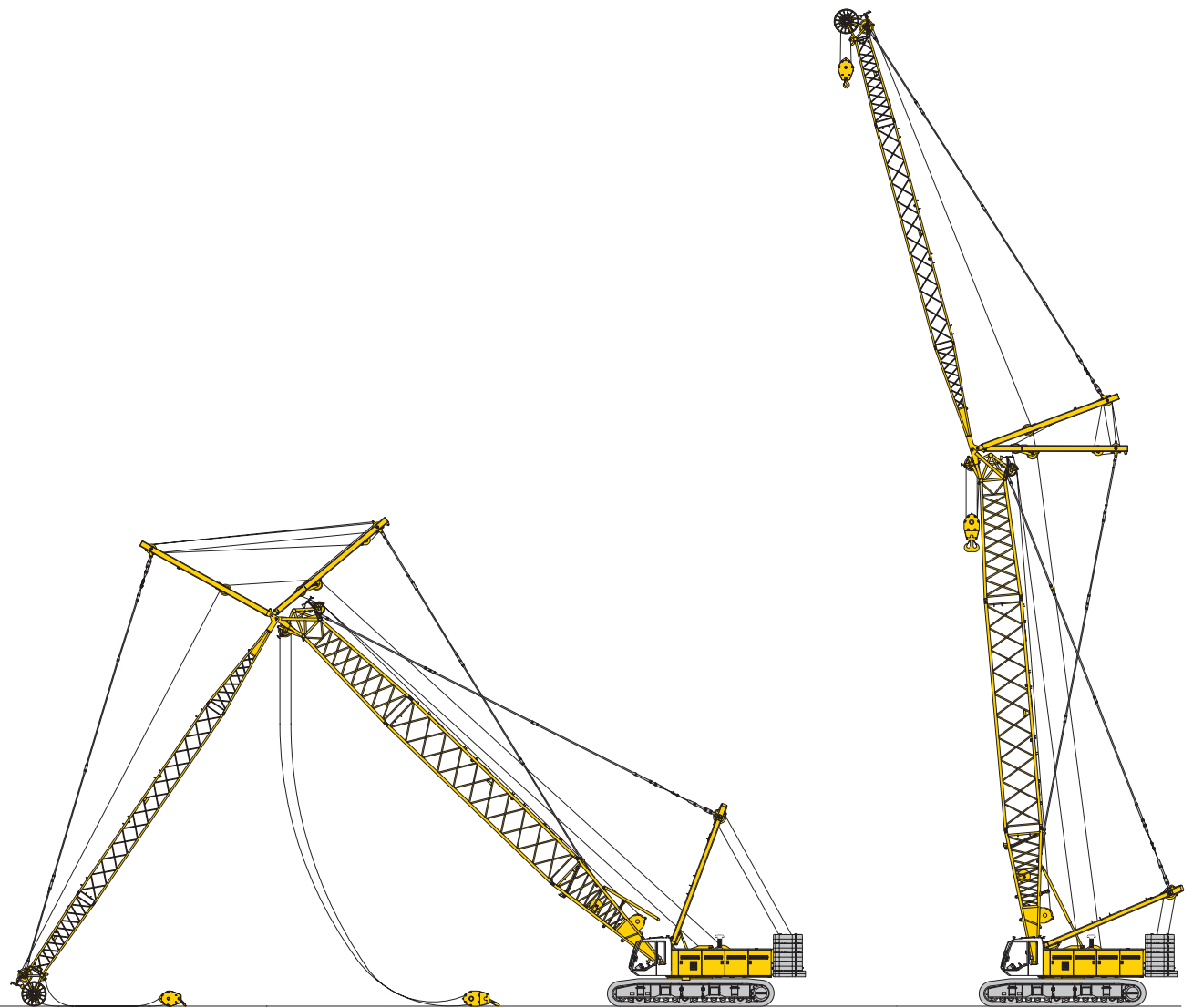
Erecting of main boom and luffing jib
